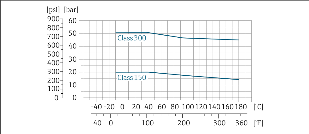
38 Process connection material: carbon steel, A105
