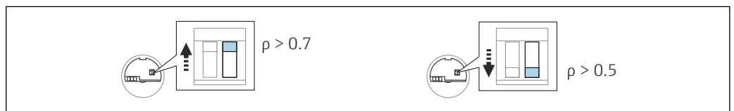
45 Switch position on the electronic insert for density
